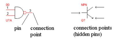
Connections to the symbol should be via the pins on the symbol. All connections should be made at the end of the pins, otherwise it will not be considered connected by the Special tools. Sometimes the pins are hidden. In this case the connection point will be obvious by the design of the symbol. For example, the npn transistor has no visible pins, connection to this symbol is via the two diagonal lines of the collector and emitter and the straight line of the base.
